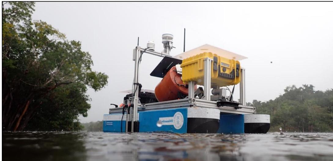
Figure 1. The platform on Jandira Lake, Amazonas, Brazil; Chamber system in flushing position.
