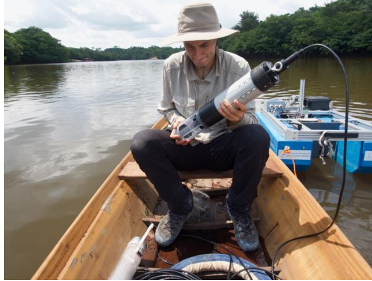
Figure 2. The multiparameter probe ready for a hydrographic profile
