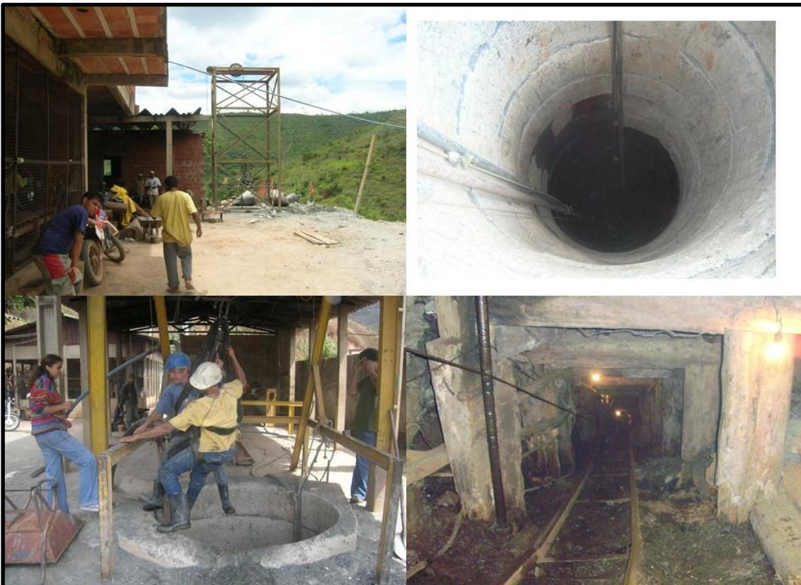
**Figura 6.** Some aspects of the region. a. Production plant with shaft structure; b. Principal shaft of 80m; c. Transport of workers into the mine; d. Production gallery inside the mine.
