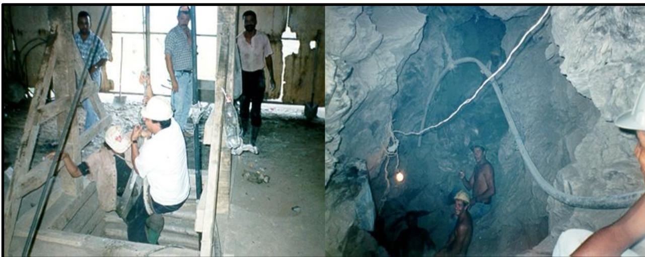
**Figure 20.** a. Mouth of the shaft of Carnaíba mine. b. End of an exploitation gallery with workers and equipment. At the mining front, concentrated emerald crystals in the host rock can be seen.
